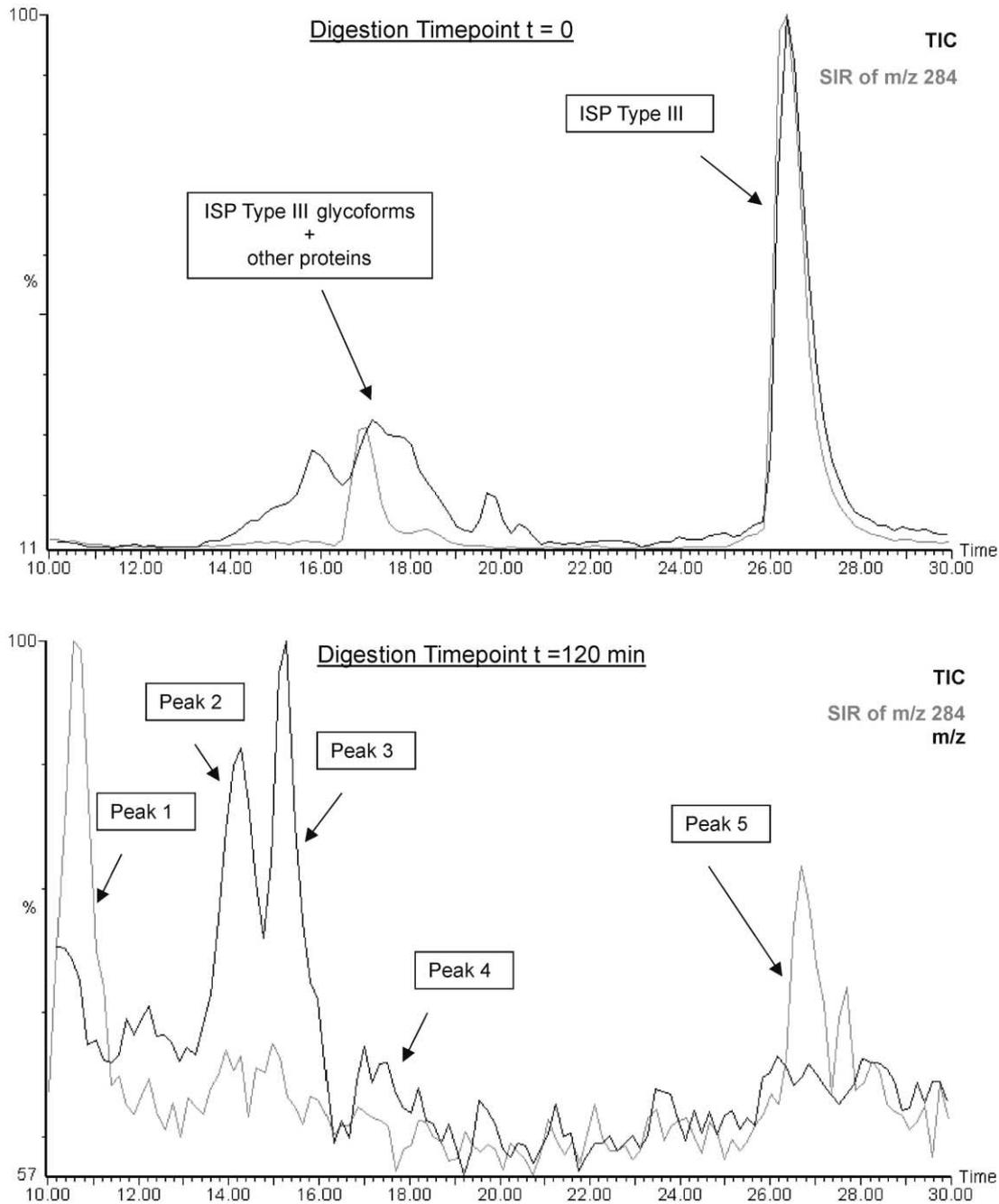
Fig. 6. Combined mass spectra extracted tic after 120 min of digestion.
